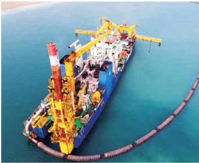
In January 2010, the cutter suction dredger “Sky Whale”, invested and developed by CCCG (China Communications Construction Group) while built by CMGL (China Merchants Group Limited), was brought into service. “Sky Whale” ranks the first in its technical capability and dredging capacity in Asia. As one of the three biggest self-propelled dredgers of the world, it is able to excavate 4500 cubic meters of seabed mixtures. The picture shows “Sky Whale” working on the sea.
